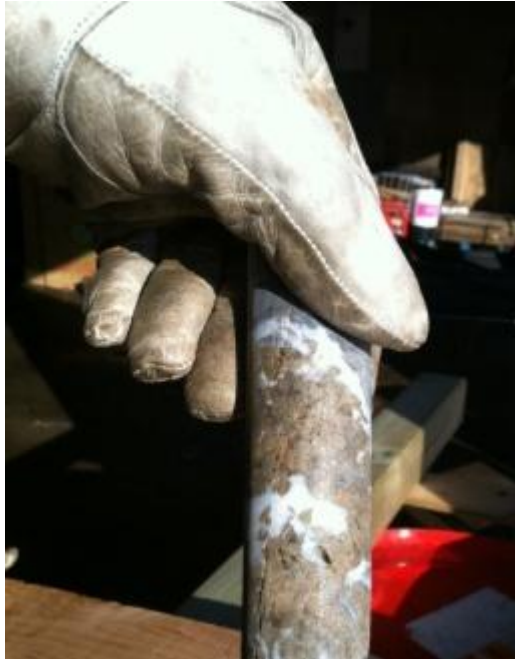
Figure 5: Sphalerite (zinc sulphide) mineralisation in SB017 drilled at Sortebjerg.
