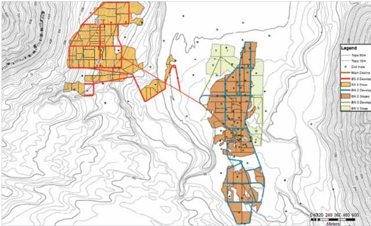
FIGURE 6: CONCEPTUAL PLAN VIEW OF THE UNDERGROUND MINE DEVELOPMENT
