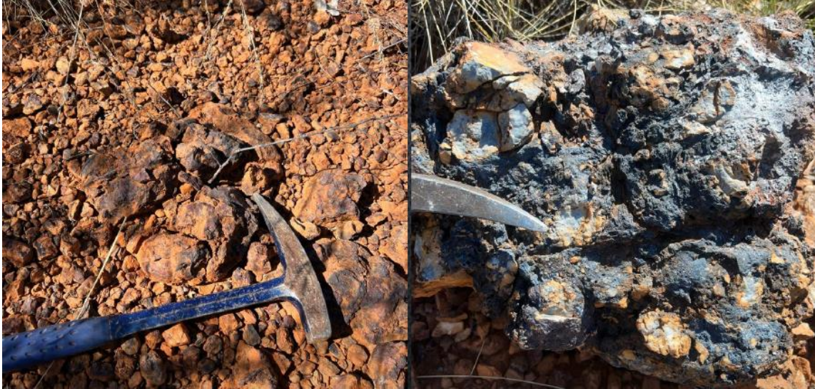
Figure 3 – Rock chip HT018 (left) and HT019 (right). HT018 returned a reading of 2,977ppm Cu and HT019 was 544ppm Cu.
