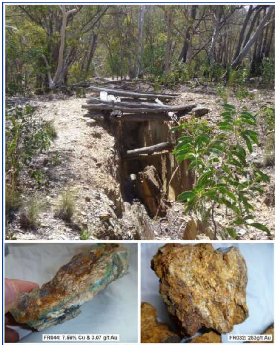
Figure 3: TOP- Photograph of one of the many historic workings at the Fiery Creek Prospect. LOWER LEFT- Sample FR044: a malachite and azurite mineralised schist containing 7.56% copper and 3.07 g/t gold. LOWER RIGHT- Sample FR032: oxidised mullock sample from the Fiery Creek workings containing 253g/t gold
